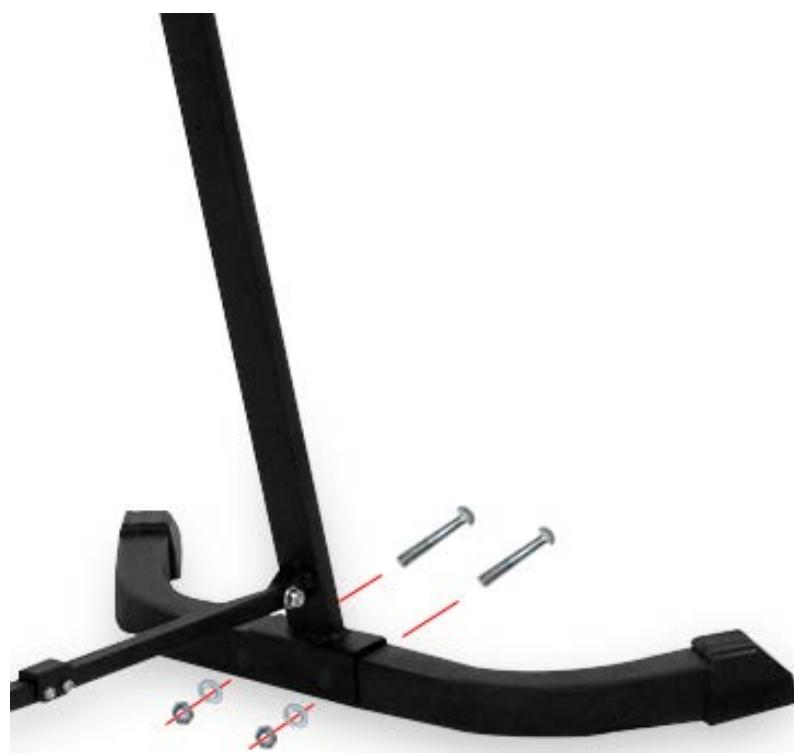
Place the rear foot tube (30) below of the support frame (2). Make sure the foot tips point backwards. Attach both parts with 2x screw, flat washer and nut.
