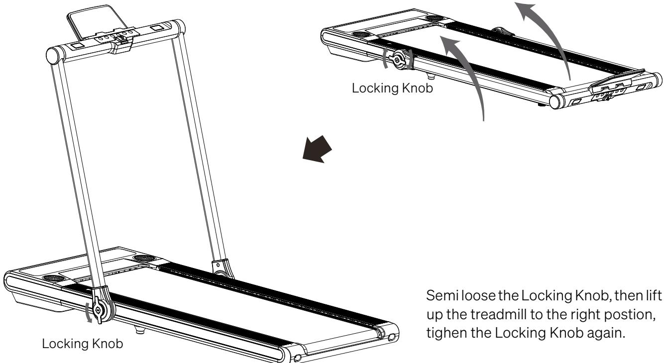
Semi loose the Locking Knob, then lift up the treadmill to the right postion, tighthen the Locking Knob again.
