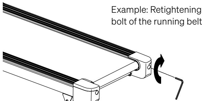
Example: Retightening the right-hand bolt of the running belt
