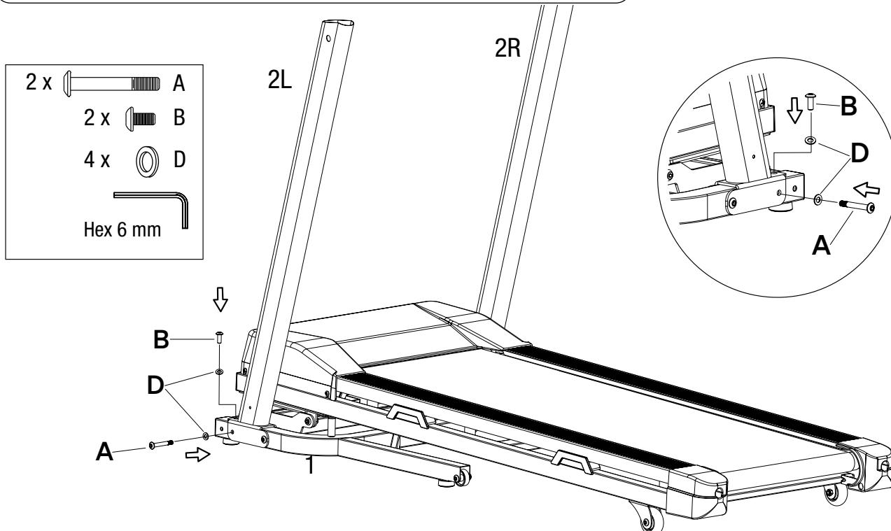
The console stands (**2L** and **2R**) are pre-assembled to the base frame (**1**).
